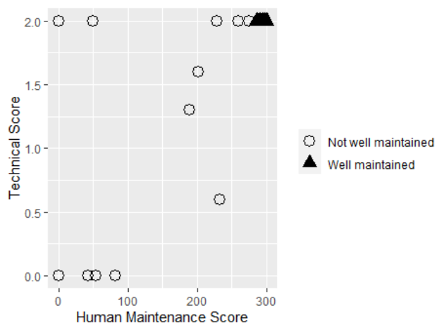
Fig. 2. The technical score plotted against the human-maintenance score for both well-maintained and not well-maintained fences (as determined through the blind assessment).
