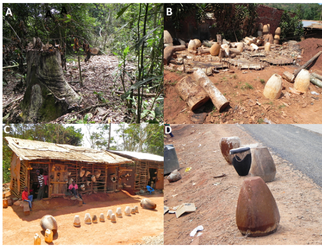
Fig. 2. Stages of drum making in Mpanga Central Forest Reserve near Mpigi, Uganda. (A) Felling of trees (which is contrary to forest regulations), resulting in a large stump (foreground), and a fallen log (background). Most of this tree has been cut up and chipped out to make blank drums. (B) A drum-making yard showing sectioned logs used as raw material (foreground) and drums in various stages of manufacture (background). (C) Finished drums and other handicrafts for sale in roadside stalls. (D) Close-up view of finished drums.
