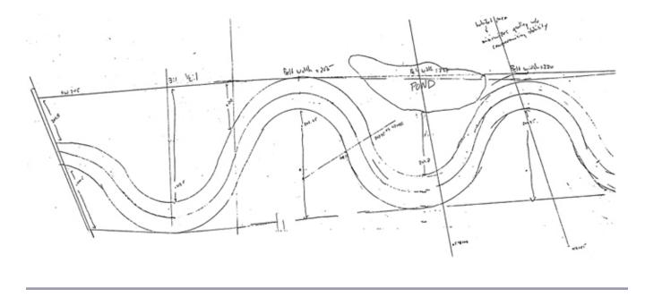
**Fig. 7**. Plan for channel reconstruction, Uvas Creek, prepared by consultants (Source: Uvas Creek project files, City of Gilroy, California).
